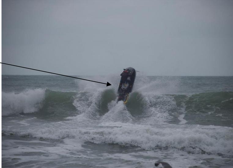
Try to keep craft perpendicular to wave and whitewater, this will allow for the best penetration through it. This will also help to avoid capsizing the craft.
